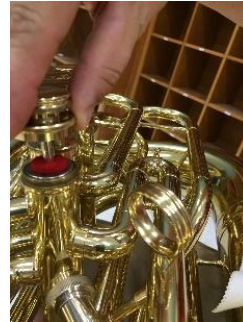
Putting valve back into position
